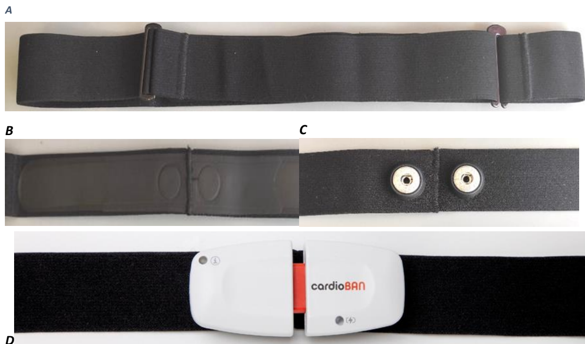
Figure 10: Chest strap (A) with dry electrodes (B) and snaps (C) to connect to cardioBAN (D).
