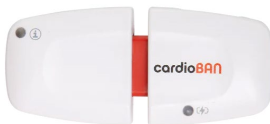
Figure 2 - CardioBAN front view. This wearable is used to measure Electrocardiogram and extract HR, HRV. Movement is also detected via an accelerometer sensor.
