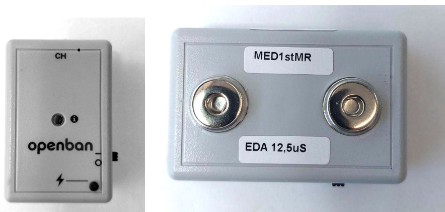
Figure 4 - EDA wearable front view. Back view with the metallic snaps for the Gelled electrodes.
