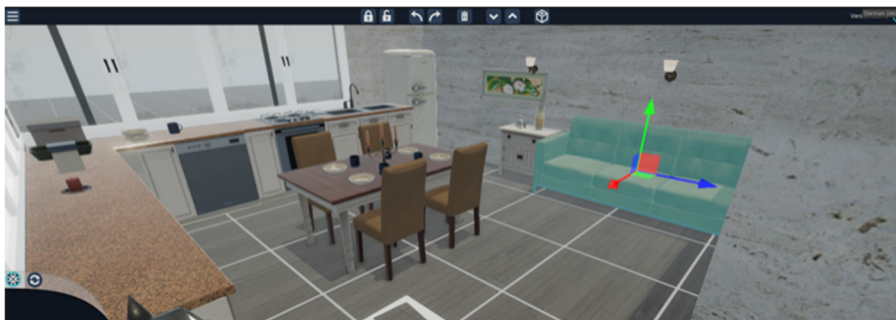
Figure 18: Positioning virtual object by handles for x-, y- and z-axis.
